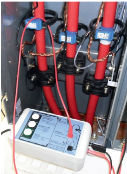
Connection of current output to CTs
