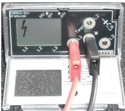
Connection of voltage output to CAPDIS
